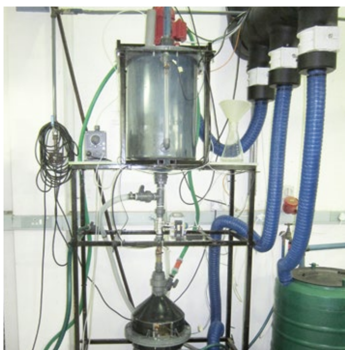
Figure 2: The automated struvite precipitation plant at the Pollution Research Group's laboratory (UKZN) doses the exact amount of magnesium and urine.
