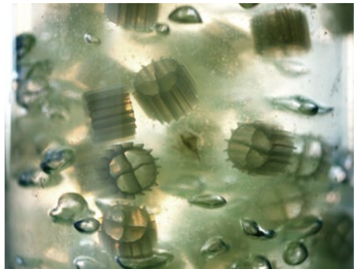
Figure 1: Plastic biomass carriers provide support for the nitrification bacteria.
