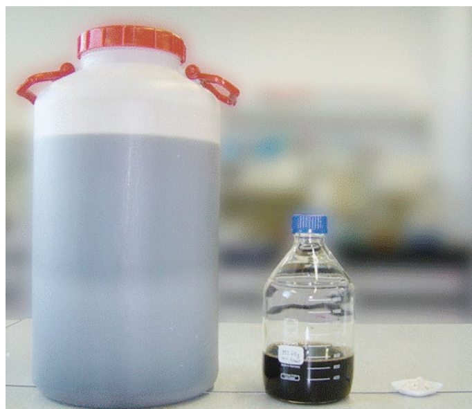
Figure 3: About 800 mL of concentrate or 600 g of dry solids can be produced from 20 L of nitrified urine.
