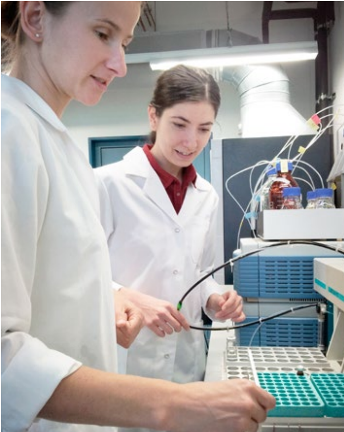
Figure 2: Measuring pharmaceuticals with solid phase extraction (SPE) coupled to liquid chromatography with tandem mass spectrometry (LC/MS/MS).
