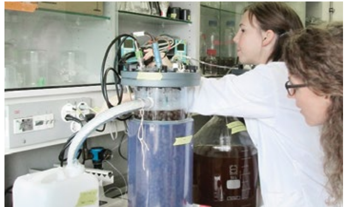
Figure 3: Studying how the nitrification reactor inactivates bacteria and viruses.
