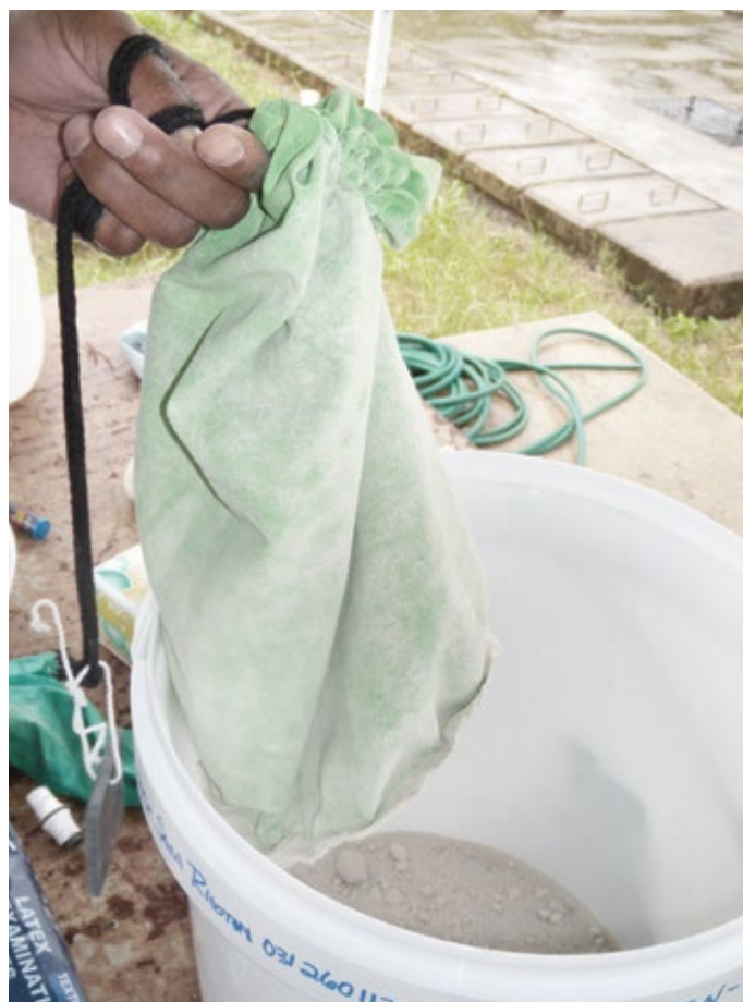
Figure 3: Producing struvite at the field test site in eThekweni.
