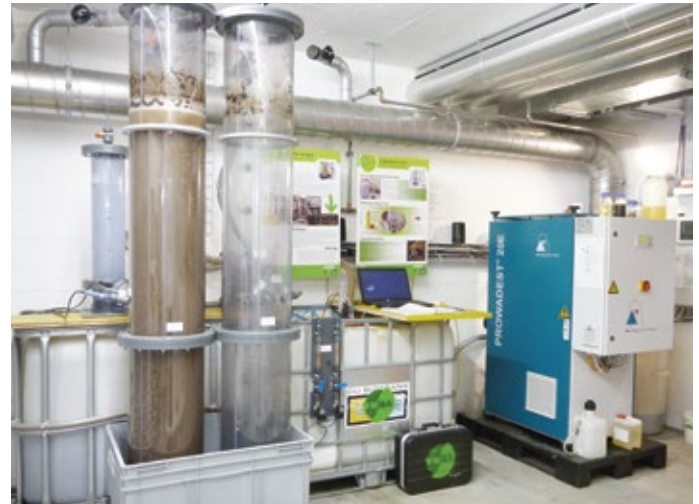
Figure 2: Complete nutrient recovery—one of three nutrient recovery plants built by the VUNA Project operates in Eawag’s basement. The two other plants recover nutrients from urine in Durban.
