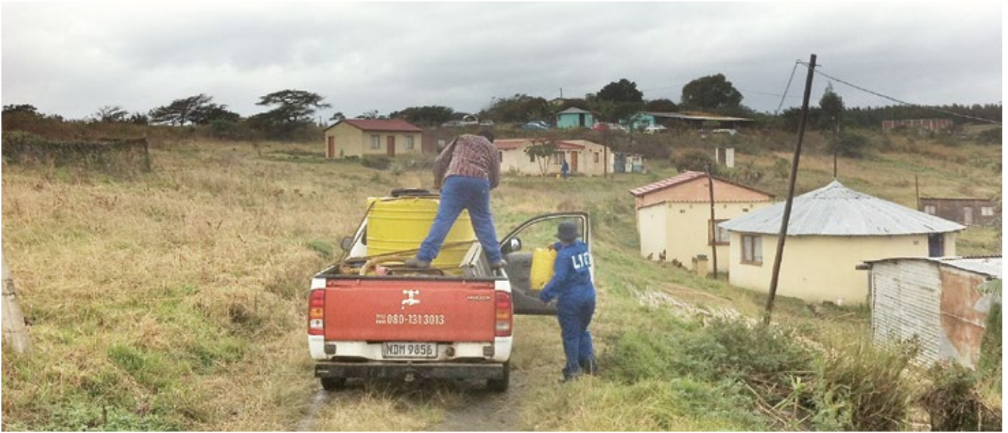
Urine collectors transfer urine from a jerry can into the collection tank on their truck.
