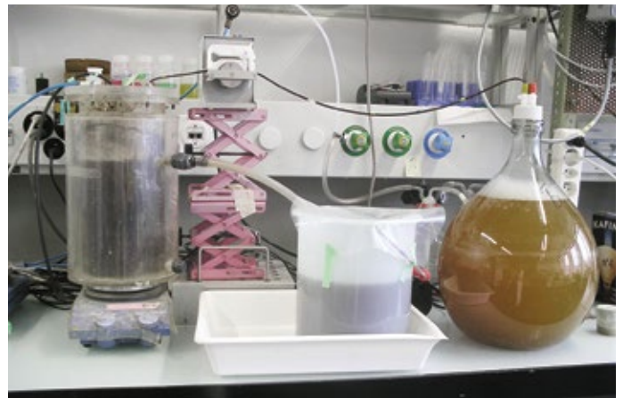
Figure 4: In a laboratory scale nitrification plant, we determined how ammonia, nitrite, and pH influence the activity of ammonia-oxidising and nitrite-oxidising bacteria.
