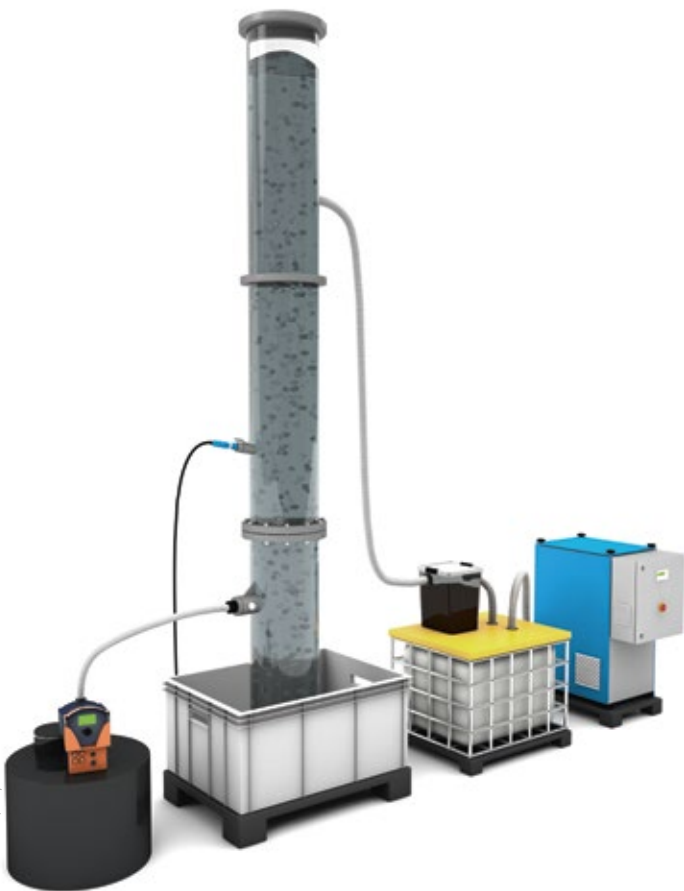
Figure 2: Bacteria in an aerated column stabilise the urine before the liquid is evaporated in a distiller.
