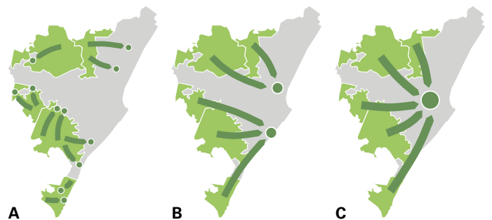
Figure 1: The business model examined different urine collection scenarios at various scales: A) twelve small decentralised urine treatment plants; B) two medium centralised treatment plants; C) one large centralised treatment plant.
