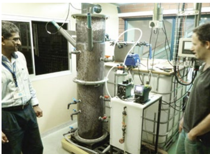
Figure 3: eThekweni’s Customer Care Centre in Durban produces its own fertiliser from urine.
