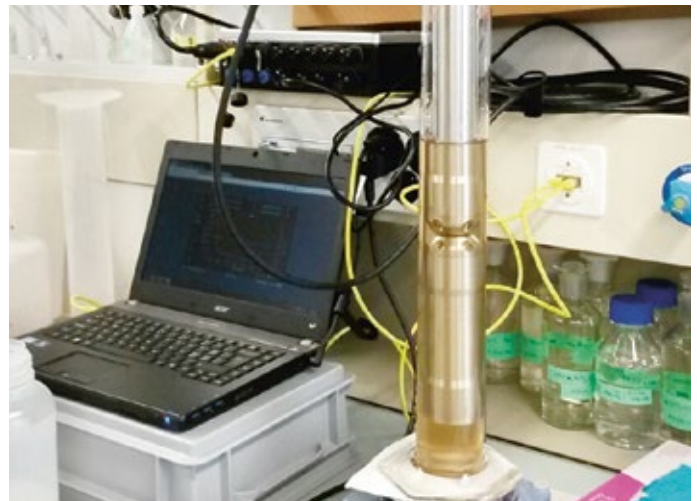
Figure 4: The nitrite concentration in urine can be estimated using an ultraviolet spectral probe. Before we tested the probe on the urine nitrification plant, we had to carefully calibrate it in the laboratory.
