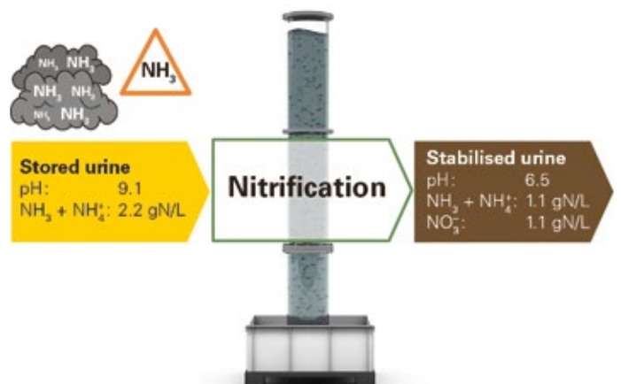
Figure 1: Nitrification lowers the pH in urine, preventing ammonia from volatilising.
