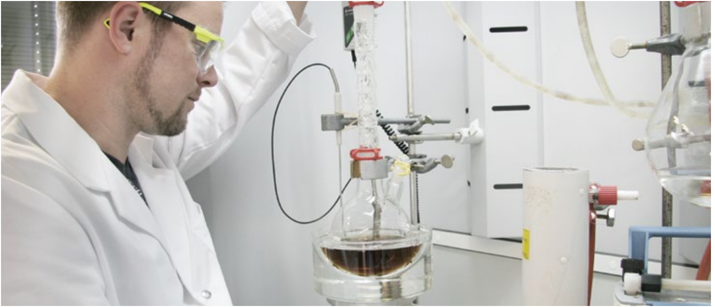
Distillation experiments in the laboratory investigated how salts precipitate in nitrified urine.
