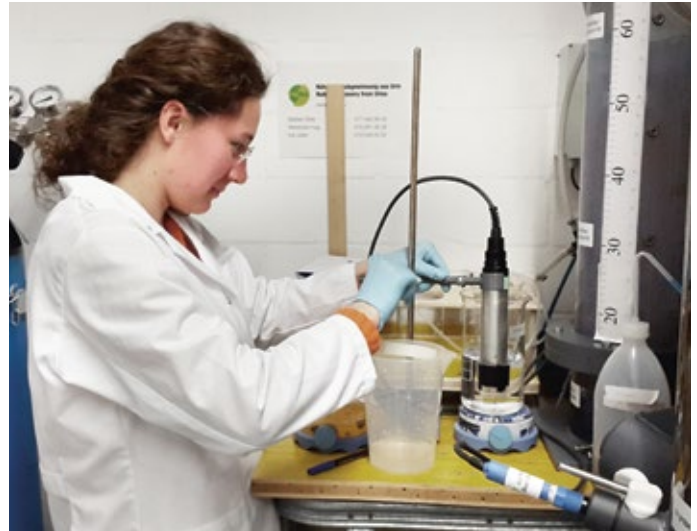
Figure 3: To precisely measure pH and dissolved oxygen, we had to evaluate the sensors' response to changing conditions. Based on the real-time measurements, we were able to estimate the nitrite concentration in urine.
